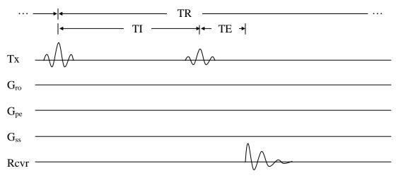
We'll start with a simple inversion recovery experiment (no imaging gradients):
