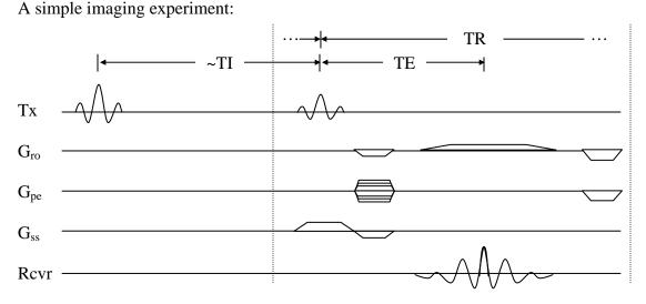
\*Note that we've pulled the inversion pulse (the magnetization preparation) outside of the imaging loop. If we can get the entire image acquired on a time frame that is small relative to the  $T_1$ 's, then the  $T_1$  contrast is the same throughout the image and we only needed one 180° pulse.
